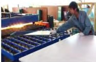
Heated roller press will compress the IGU.
