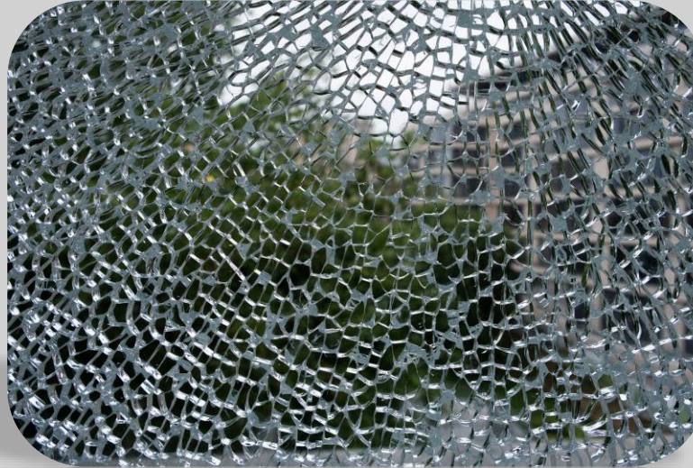
Fully tempered glass Resistant to breakage; four times as strong as annealed glass; shatters completely in small pieces, typically vacating the frame after impact
