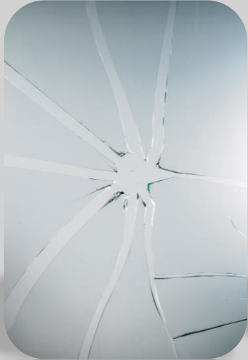
Annealed glass Breaks easily, typically in long, sharp shards
