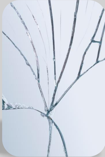
Heat-strengthened glass Resistant to breakage; two times as strong as annealed glass; Breaks in large shards
